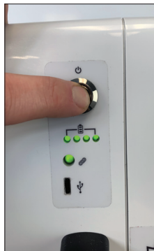
FIGURE 6: PROP CONNECTED AND INDICATING FULL POWER
