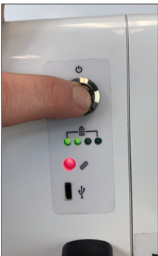
FIGURE 5: POWERING ON PROP
