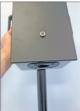
FIGURE 2: PLACING PROP BOX ONTO TRIPOD
